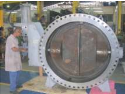
Butterfly Tri Eccentric Valve Test
