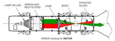
As shown here the green and red light beams are refracted by the water present in the port and captured by the frosted glass in BRIGHT GREEN.
